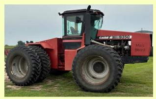
Case-IH 9350 4WD, Quad Range, Cummins M-11, 4 Hyd., Good 520/85/42 Rubber, New A/C, 6037 Hours, SN-JEEO071696
